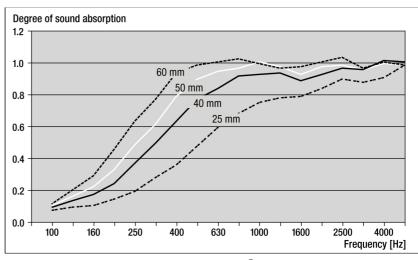
Diagram 4: Degree of sound absorption of Basotect® G+ as a function of the thickness, according to DIN EN ISO 354 (reverberation room)
