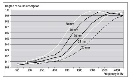
*Diagram 3*: Degree of sound absorption of Basotect® G+ as a function of the thickness, according to DIN EN ISO 10534-2 (impedance tube).
