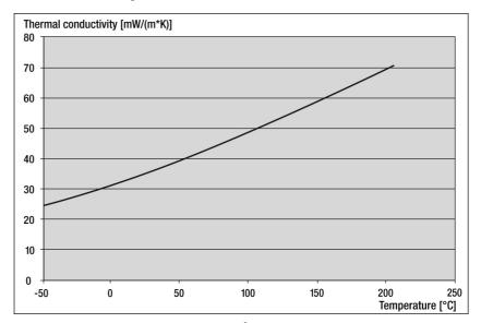
Diagram 2: Thermal conductivity of Basotect® G+.
